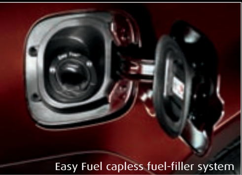
Easy Fuel capless fuel-filler system
