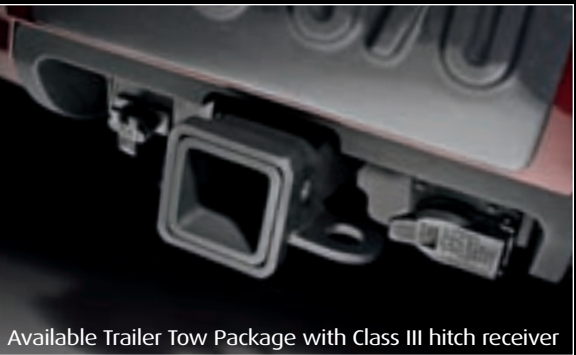
Available Trailer Tow Package with Class III hitch receiver
